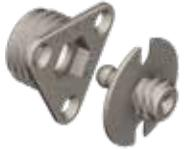
The Metal Range is recommended for more heavy duty applications that require a robust hidden fixing with the innate fire resistance of metal. Self-tapping, screw or rivet and self-adhesive fix options available, with pull-out loads of 5kg or 10kg depending on female clip used. Common uses: heavyweight wall and ceiling panels, fire-rated panels, metal panels.
